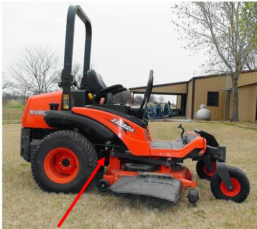
Similar Kubota ZD series Mower- PIN plate on right frame under fender, inset from right rear wheel
