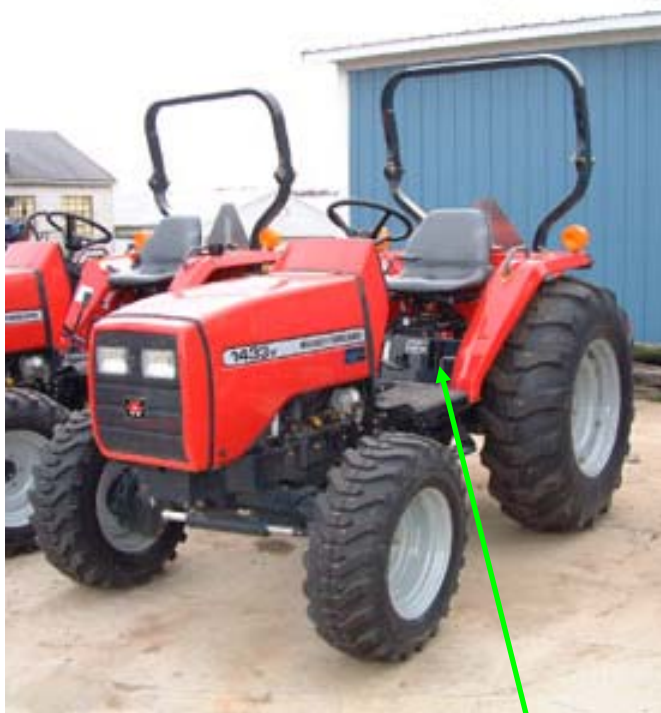
Image of similar machine. PIN decal or plate located below drivers seat
