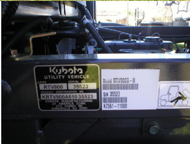
Kubota RTV-900 PIN Location- PIN is visible with bed in lowered position
